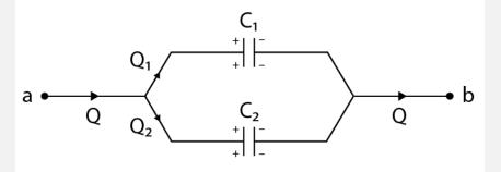
The ratio Q/V is called the equivalent capacitance C between points a and b.
