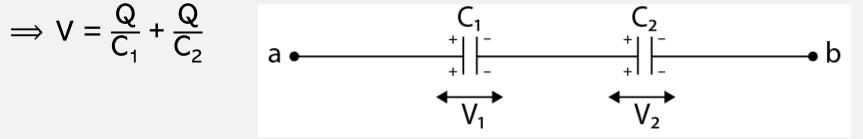
The ratio Q/V is called the equivalent capacitance C between points a and b. The equivalent capacitance C is given by:  $\frac{1}{C} = \frac{1}{C} + \frac{1}{C}$
