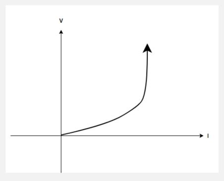
Examples of non-ohmic resistances are diodes, SCRs (Silicon controlled resistors), transistors, etc. Voltage is no more proportional to current. The relationship between V and I is not unique, which means, more than one value of voltage is obtained for one value of current.
