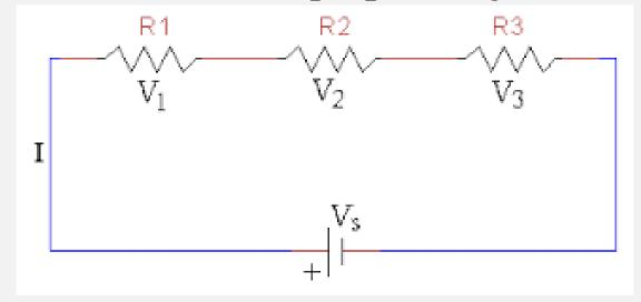
Effective resistance,  $R = R_1 + R_2 + R_3$
