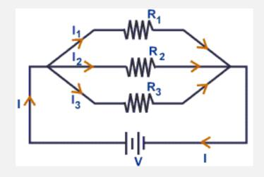
Effective resistance,  $\frac{1}{R} = \frac{1}{R_1} + \frac{1}{R_2} + \frac{1}{R_3}$ The current through the combination,  $I = I_1 + I_2 + I_3$ The voltage remains same.
