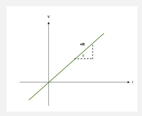
Linear V-I characteristics are shown by ohmic resistors. The slope of the line gives resistance. Higher the slope, the higher will be the resistance.
